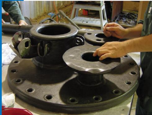
reinforced stocks. These compounds are formulated for services involving wet chlorine, strong acids at high operating temperatures, plating solutions and water conditioning equipment. All have a soft tie gum for maximum adhesion to steel.
